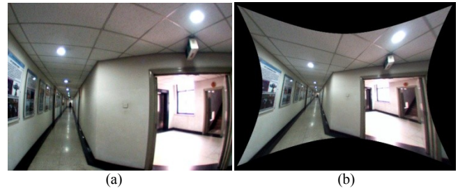
Fig. 6. (a) A real image of a corridor with radial distortion. (b) The corrected image from (a).
